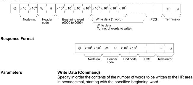
**Note** If data is specified for writing which exceeds the allowable range, an error will be generated and the writing operation will not be executed. If, for example, 98 is specified as the beginning word for writing, and three words of data are specified, then 100 will become the last word for writing data, and the command will not be executed because HR 100 is beyond area boundary.
